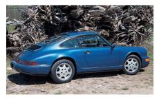
In standard form for the first three years of production the Carrera 4 used these new seven-spoke alloy wheels, with 205/55front tires and 225/50 rear tires. Considerable road noise was transmitted into the cabin because tire pressures were high.
