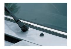
The wipers on the 911 had changed for 1968 so that they always parked in front of the driver, whether the car was left-hand or right-hand drive. Since then, the 911 designers have not been able to change the wiper arrangement significantly through the entire life of the model because of the cost of retooling.
