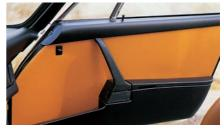
The door trim on the 1974 models received another revision. The rear compartment was now deeper and had a conventionally hinged top lid to replace the elastic bungee sprung "clamshell" of the previous design.
