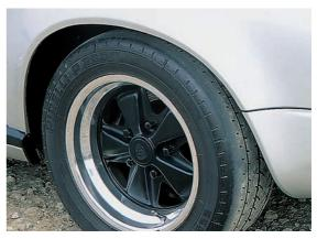
By 1975, the Fuchs forged-alloy wheel had become the required fitting. From the early narrow examples, changes had centered on increasing the wheel width and improving the finish of the rim. The RS had introduced different front/rear wheel sizes, and this practice was carried over to the later 2.7 Carreras. This is a rear 7Jx15 wheel with a nonstandard 225/50 tire.
