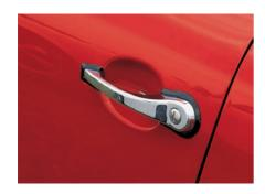
For 1970, there was another revised exterior door handle with the introduction of the definitive hidden trigger-release. Door operation now had to be a deliberate activity with no possibility of accidental opening. The keyhole was given a hinged cover, which reduced the possibility of the lock freezing up.
