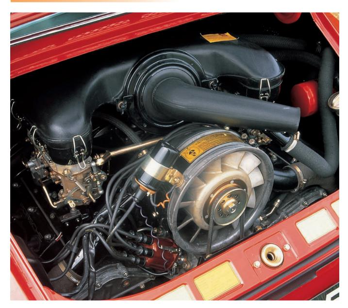
The European 2.2T used two triple-choke Zenith TIN 40 carburetors. The oil filler neck is on the right-hand side with the oil filter just behind.
