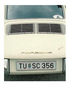
Rear view of an Austrian 911 (above) shows the complexity of the hand-assembled engine lid grille of the 2-liter cars. The manufacturing cost of the grille was later reduced by using pressed bars and welded construction. The 1967 911S (above right) shows the rubber trim introduced on the rear over-riders for this model year. These items were previously in plain chrome. This model year was the last when the engine cover featured a distinctive central body rib under the grille.
