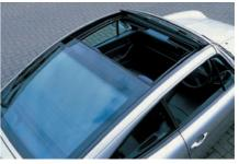
The Targa's roof was thermally insulated and filtered ultra-violet light. The elegance of the design is evident, particularly in the absence of the old rain gutters of the coupe and the new form of the rear side window. The opening glass slid back under the rear window at the touch of a switch to provide open-air motoring. The panel in front of the sliding roof opened forward to prevent wind buffeting inside the car.
