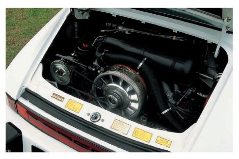
Rest-of-the-World models retained the air-injection pump, seen here on the left of this 1982 engine compartment. The air filter for the pump can be seen behind it, with a red wing nut on top. After a brief period when a five-blade cooling fan had been used, the SC returned to an 11-blade version. This fan and many of the fittings around the engine have been highly polished, to good effect.
