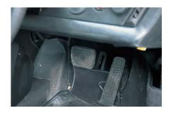
By 1979, when this car was built, the two-pedal Sportomatic transmission was available only on special order. This novel but halfway house automatic shift was deleted the following year.
