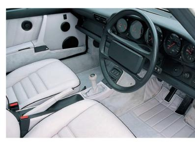
Apart from new trim choices and door loudspeakers, the only significant change in this Carrera 4's interior architecture compared with the old Carrera 3.2 is the higher central tunnel necessary for the four-wheel-drive system.
