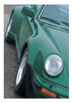
The wide wings on this 1976 model housed big 7Jx15 front and 8Jx15 rear Fuchs wheels and spacers increased the track. The tires on these first Turbos were usually Pirelli CN36s with 185/70 front and 215/60 rear sizes, which met U.S. bumper height requirements.
