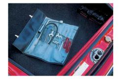
The 1968 S had a soft-grain finish to its tool bag, but from 1969 the tool bag vinyl changed to a basketweave. The chassis number plate is seen to the left of the latch, with the windshield washer filler on the right. The battery at top right has the correct rubber strap and plastic cover.
