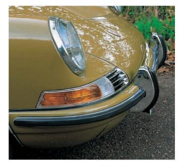
This 1971 S has the correct nonfrosted top edge to its Bosch H1 headlamp glass. From 1973, the top edge was frosted and many owners retrofitted the simpler single-bulb H4 unit.
