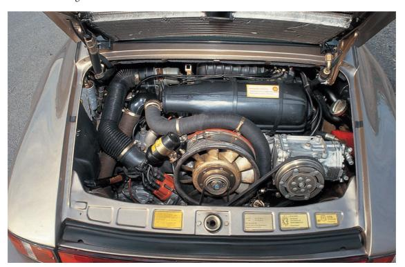
A busy engine compartment on this Californianspecification 1980 911SC, with the air conditioning compressor (and revised condenser coil) on the right. This was the first year the SC was not fitted with an airinjection pump: This was replaced by a sensor that measured the oxygen in the exhaust and was linked to the fuelinjection system.
