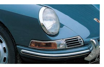
The earliest style of horn grille was made of chrome-plated brass and mounted with four screws (above), but a cheaper design for the 1967 model year was secured by only two screws (below). Both cars have the European-specification Bosch asymmetric (nonsealed-beam) headlights used until the end of the 1967 model year, but the bumper styles differ because the later car, without over-riders, has the wide rubber insert that was a new feature of the S.
