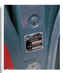
The chassis number on early models is found on the left-hand door pillar. Also shown on the plate is the paint code (Farbton) 6401, Slate Gray.
