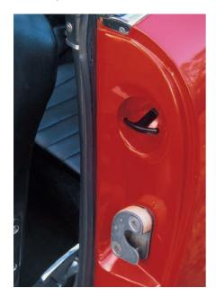
The engine lid release on the 911 is to be found on the left-hand B pillar. This feature is not so convenient for right-hand drive.
