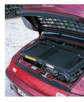
There is an engine under there somewhere! Twin air-to-air intercoolers dominated the engine compartment of the Turbo.
