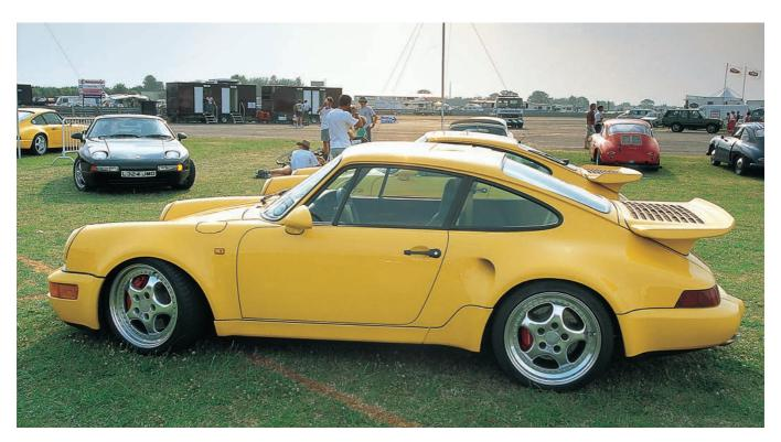
The 1987 Turbo Slant-Nose derived its front profile from the 935 racer, but pop-up headlamps were added. Early customized Slant-Nose cars lacked pop-up headlamps, having the lights mounted below the bumper line.
