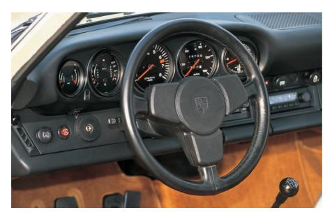
The 1974 Carrera retained the 380-millimeter steering wheel of the RS. The new side vent in the lower dash greatly improved side window demisting. The redline on the rev counter starts at 6,300 rpm and shows that this model was no RS. The latter was redlined at 7,200 rpm.
