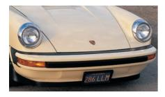
By a superbly clever mix of design and function, Porsche's stylists turned a potentially disfiguring legal requirement for energy-absorbing bumpers into an image-enhancing feature. Just visible here is the flexible lip extension to the new front spoiler, an important detail that improved the aerodynamic balance of the car when the rear ducktail was fitted.
