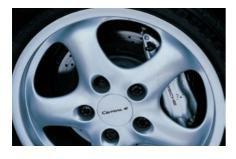
The brakes on the 993 were outstanding, featuring cross-drilled and ventilated discs and four-piston calipers. ABS 5 helped ensure the wheels did not lock up when the pedal was pressed too hard.
