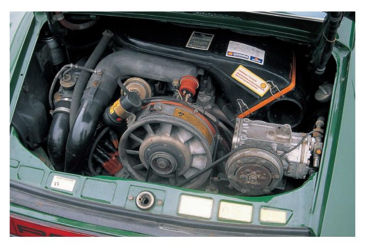
The previous model's early Motronic injection ignition system was retained. Compared with the 3.3-liter engine, the compression ratio was increased from 7.0:1 to 7.5:1, and maximum boost went up to 0.85 bar. Power rose from 320-brake horsepower to 360-brake horsepower, and Porsche claimed fuel consumption was unchanged, if not better.
