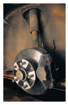
Club Sports had (green) Bilstein gas dampers as standard. All Carrera 3.2s were given larger versions of the familiar A-type cast-iron calipers and the brake discs were thicker (at 24 millimeters) than those on the SC.
