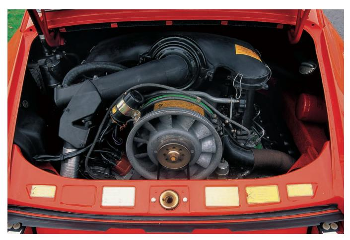
For the 2.4 models the engine air intake ducting was revised to incorporate a cold-start flap, with the opening moved from the right-hand to the left-hand side of the engine compartment. When the engine was cold, the flap prevented ambient air entering the intake ducting, and warm air was drawn from around the left-hand heat exchanger.
