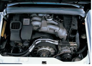
The 3. 6-liter engine gained another 22-brake horsepower. Despite weighing an extra 20 kilograms, the 993 delivered better all-round performance than the 964. The improved 1996 models (left) used a Varioram induction system and larger valves to produce 285-brake horsepower from the last full-scale production version of the air-cooled boxer "six."
