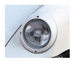
By 1986 the sealed-beam Hella headlamps fitted to U.S. cars were available with the more powerful H4 filaments.
