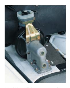
The addition of a brake servo was a significant improvement for the 911 SC. Its effect was most noticeable around town when the discs were cold. The bulk of the assembly seriously reduced the usefulness of the luggage compartment.
