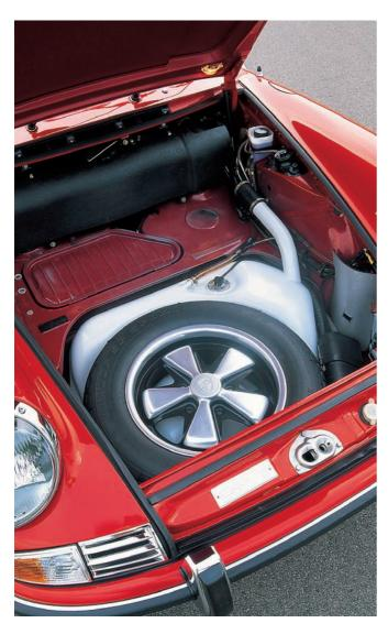
The hinged panel behind the fuel tank covered the steering joints and the location for the optional petrol heater. The brake master cylinder was moved out of this compartment and up onto the left wing wall for the 1968 model year, when dual-circuit braking was introduced. The fuse box, larger than before, has been moved to just behind the left-hand battery.
