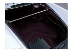
The tidy luggage compartment of a 1986 U.S. Turbo (above): The aftermarket brace between the tops of the MacPherson struts is a well-proven modification to stiffen the front structure of a 911, thereby reducing wheel camber change during hard cornering. When stripped of its carpets (below), the luggage compartment of the 3.6 Turbo shows how carefully every component has been packaged. The front strut brace is now standard.
