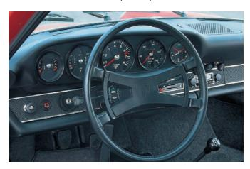
The instrument panel on a 1971 T, showing only detail changes: the hazard warning flasher button, introduced in 1970, is on the left-hand lower dash, and there are improved switches with large rubber surrounds. The labeling behind the steering wheel indicates headlamp flash and turn signal operation but is completely obscured from the driver!
