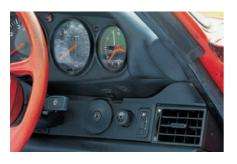
The ventilation system was improved again for the 1986 model year, with larger face level and side window vents. The headlamp level adjustment was introduced for 1987. The nonstandard slot next to the sunroof rocker switch is the keyhole for an aftermarket engine immobilizer.
