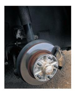
The front suspension of this 1965 car shows the MacPherson strut and, behind it, the actuating lever for the 13-millimeter anti-roll bar—an early attempt to stiffen the front and delay the onset of oversteer. Brake discs were solid and at the front used the M-type cast-iron caliper.
