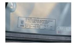
This factory label shows that the 911SC was comfortably within Californian emissions limits for hydrocarbons, carbon monoxide, and oxides of nitrogen.
