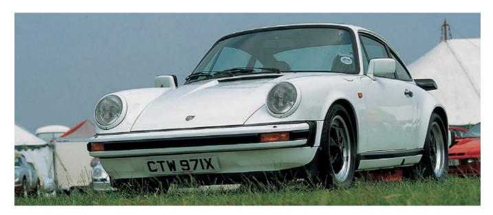
Bilstein dampers gave a firmer ride, and special Fuchs wheels with Platinum Metallic centers were used irrespective of body color. These wheels were fitted with Pirelli CN36 tires of sizes 185/70VR15 front and 215/60VR15 rear, on 6-inch and 7-inch rims, respectively. Other decorations included a passenger door mirror, electric sunroof, foglights below the front bumper, and an electric aerial with speakers fitted in the doors and on the rear shelf.
