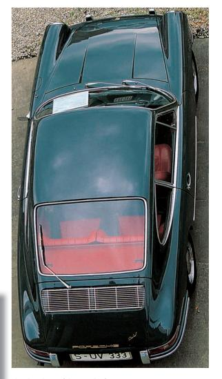
The clean lines of the Porsche factory's own 1964 911 coupe. The first 911s had minimal flaring to their wings, giving the cars a clean aerodynamic shape. Evident in this view is the Durant driver's door mirror of 356 vintage.
