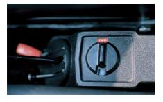
A new option for 1976, and standard on the 3-liter Carrera, was automatic regulation of cabin temperature. A controller was fitted between the seats and monitored inputs from sensors. The controller drove a servo motor that opened or closed butterfly valves on the heat exchangers.
