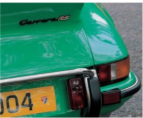
Rear ends of an M472 RS Touring (above) and an early M471 RS Sport (below). The Touring has steel bumpers, a nudge bar, a chromed silencer skirt, and a molded badge under the ducktail. The Sport has a one-piece glass-fiber "bumper," the engine lid is secured with racing-style elastic toggles, and the badges are color-coded decals.
