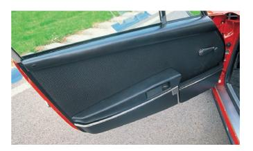
New door trims were introduced for the 2.2 models. Their features were rigid storage pockets (the rear one hinged outward) and a recessed door handle lever—much safer than the previous push-button release.
