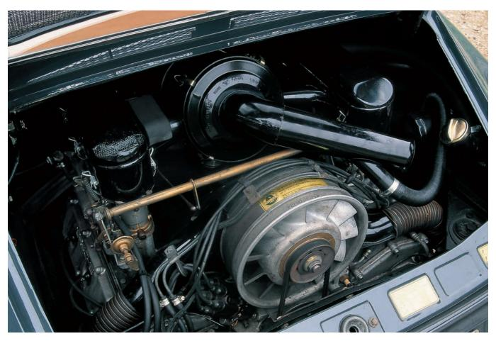
The vertically mounted fan distributed cooling air to the cylinder barrels more evenly than the 356's axial unit. The Solex overflow carburetors seen on each side of the engine were difficult to tune correctly and gave the engine a significant flat spot around 2,500 rpm. The later label (mentioning the 911S/911L) on the fan housing is incorrect on this 1965 model.
