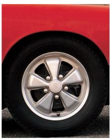
The classic Fuchs forged-alloy wheel was introduced on the 1967 model year 9115, but the narrow rim width of 4.5 inches dismayed *Car and Driver* magazine. Note the restrained use of black paint on these early wheels and the elegance of the non-spoilered front profile.
