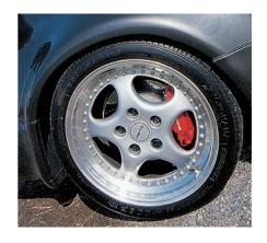
The 3.6 Turbo runs on special 18-inch Speedline wheels. The 8J front rims carry 225/40 tires and the 10J rears have 265/35 tires, an incredibly low profile.
