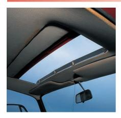
An electrically operated sunroof was an option from the start of production. The small wind deflector at the leading edge popped up as the roof was opened, inhibiting wind buffeting. The interior mirror was initially attached to the roof by three screws, but for 1968 the mounting became a "breakaway" design attached to the windshield.
