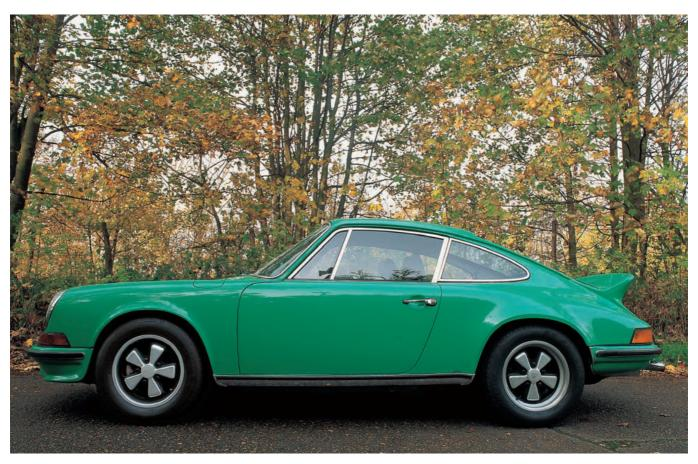
Pointing to the 911's aerodynamic future, the Carrera RS was the first model to sprout a rear spoiler, although the ducktail was actually an option.
