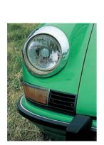
This T has the more pronounced chromed headlamp flange that goes with the sealed-beam units fitted to U.S. cars. These headlamps were unpopular, as shown by this car having the more powerful Lucas H4 units retrofitted. Also visible is the large elastomer overrider used only in 1973.
