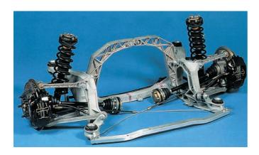
Porsche's lightweight-stable-agile (LSA) design provided the 993 with new multi-link rear suspension—a major change under the surface.
