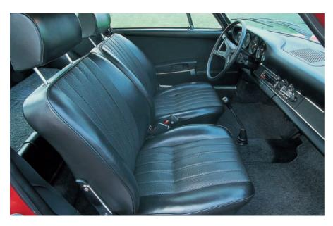
The interior of a 2.2 911 was now far removed from the early models. For the 1969 model year the lower dash had been revised to include more effective heating and ventilation controls. The ashtray was moved to the central area, the glovebox lid was further revised, and the speaker grille was now removable. From 1969, too, the seats could be tilted forward by operating a lever at the top of the seat back support, instead of down at the hinge point.
