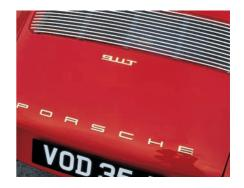
This decal appeared in the rear window of all 2.2 models. The simple chromed engine lid grille has a black-painted mesh beneath to stop objects falling into the engine compartment.
