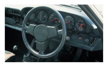
The instrument panel of the SC was little changed from the European Carrera 3.0. Points to note are the 380-millimeter steering wheel (which obscured important sections of the speedometer) and the rocker switch for the headlamp washers sited between the speedometer and the clock.
