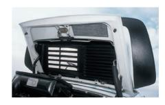
The dual functions of the tea-tray grille can be seen with the engine lid raised: The air-to-air intercooler connected into the engine intake manifold is on the left, while the air conditioning condenser on the right is mounted directly to the grille itself.
