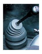
The new five-speed 915 gearbox for the 2.4 models had a conventional gear change pattern, with fifth to the right and forward. The larger gear lever boot seen here arrived for the 1973 model year.
