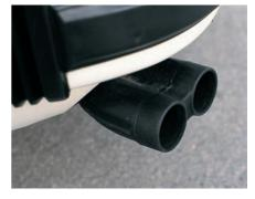
Twin exhaust tailpipes were first seen on the 1983 Turbos when the wastegate exhaust was taken directly to atmosphere.
