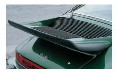
So much heat was generated in the engine compartment, particularly at standstill, that the secondary engine cooling grille was enlarged for 1976.
