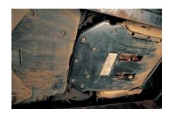
Great attention was paid to the aerodynamics of the Carrera 4. A full-length undertray to the rear of the engine not only helped airflow but also contributed to lower noise levels. Note the NACA duct below the gearbox area.
