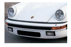
This 1986 Turbo has a replacement front air dam, complete with opening for a supplementary oil cooler and integrated mountings for driving lights.
