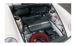
The factory said the Carrera 4 was 87 percent new under the skin, and here's some of the evidence. The luggage compartment has a completely different layout, with the plastic fuel tank now moved up and back to accommodate the front differential below, the fuse panel moved to the left-hand rear of the compartment, and the new ABS equipment under the cover to the rear of the battery.
