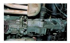
The 915 five-speed gearbox (to the right) and the exhaust pipes leading forward into the heat exchanger boxes (to the left). Air is circulated around the exhaust pipes and taken forward to warm the cabin.
