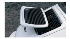
The Carrera 4 introduced an electrically operated rear spoiler (above) that deployed automatically above 50 miles per hour and retracted when speed fell below 6 miles per hour. In the wake of the Carrera 4, the Carrera 2 was introduced (below) early in 1990 to replace the old Carrera 3.2. More sporting than the fourwheel-drive model, it was modified to great effect by the factory's racing department.
