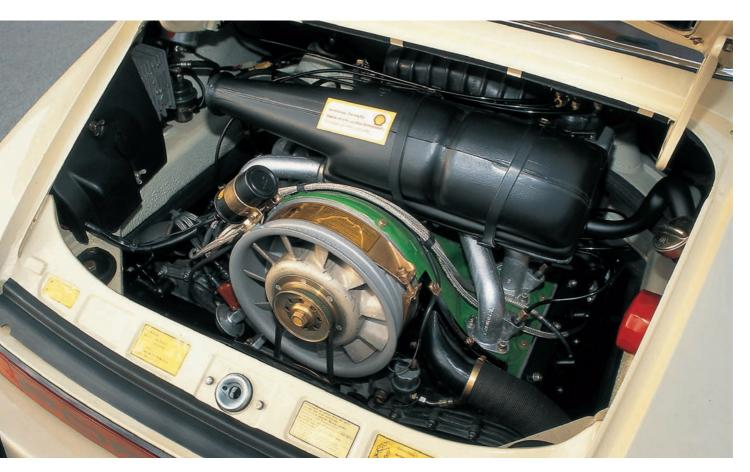
While European 1974 Carreras used the engine from the previous year's RS, U.S. models adopted that market's S engine and Bosch K-Jetronic injection. With just 175-brake horsepower, the U.S. Carreras were at a significant power disadvantage against the 210-brake horsepower Carreras offered in most other markets.
