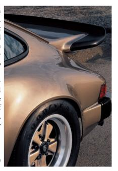
First used in series production on the 1975 Carrera, the whaletail spoiler changed in detail on the 911SC. At first the most noticeable difference was a deeper black flexible part of the assembly (above), but further revisions for 1982 meant that the center section was built up on its top surface, like the Turbo version, and the underside was cut back (below).
