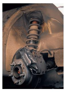
The front suspension discarded the 911's timehonored torsion bars and adopted conventional coil springs over the shock absorbers. A significant redesign of the front chassis was necessary to accommodate four-wheel drive.
