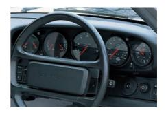
The instruments were totally updated for the new models (above). The figures and indicator needles were now backlit at night, and the oil combination gauge now contained an array of warning lights. This car does not have the air bag steering wheel. The instruments continued to be developed (below), and by 1992 the clock even carried its own complement of warning lights. The speedometer contained a shift indicator on Tiptronic models.
