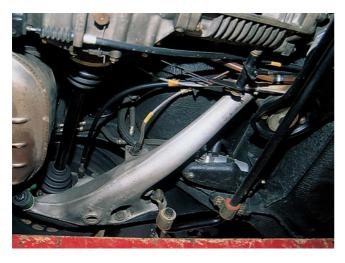
This underside view shows the forged semi-trailing arms (with embossed build date) that replaced the more flexible fabricated steel units in 1974. Other points of interest are the glimpse of the green Bilstein gas shock absorber, the fuel pump tucked away behind and above it, and the delicate mounting for the anti-roll bar.
