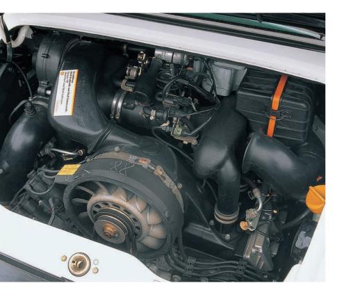
The Carrera 4 and Carrera 2 shared a new 3.6-liter engine developing 250-brake horsepower. A notable feature of the new models was the distinctive whine, like the sound of a jet aircraft turbofan, made by the revised curved-blade cooling fan while cruising.
