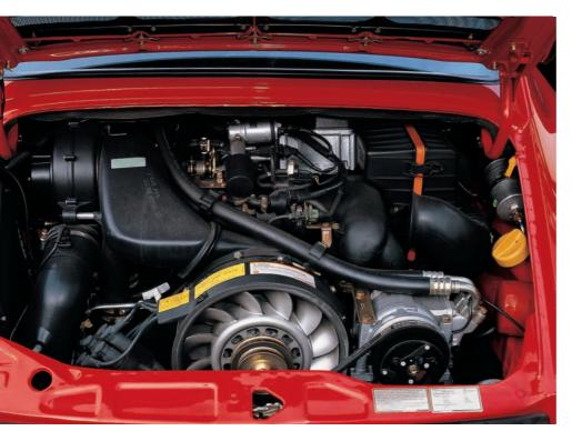
The engine of the RS America was the standard 250-brake horsepower Carrera 2 unit. Note the air conditioner compressor pipes leading directly out of the engine compartment to the remotely mounted condenser. The mechanism for the moving electric spoiler of the regular Carrera 4 and Carrera 2 models had displaced the condenser from its previous position under the engine lid grille.
