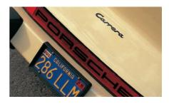
The new bumpers were neat one-piece aluminum extrusions front and rear. The rear aspect of the 911 was further changed by the addition of a full-width reflector strip between the light clusters. Possibly too flashy on some cars, it worked well on the 911. The Carrera logo had always been reserved for limited-edition high-performance models.
