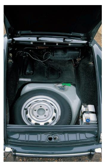
The luggage compartment, seen here on a 1965 model with the central piece of carpet removed, housed the spare wheel and the fuel tank, both of which were recessed between the front wheels to allow a useful volume on top for personal belongings. Note the fuse block fitted at the top right. The battery is attached by a later fitting, the original rubber strap and plastic cover no doubt having disappeared long ago.
