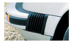
The design of the impact bumpers allowed them to move backward in a low-speed collision. Movement was resisted either by two shock absorber units or collapsible tubes fitted between the bumper and the front part of the wing inner walls. The external bellows at the sides of the bumpers were a tidy method of accommodating this potential for movement.
