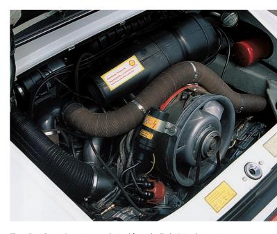
The 3-liter Carrera's engine was derived from the Turbo's, its designation changing from 911 to 930. The faster-running five-blade cooling fan is the most obvious distinguishing feature of these cars.
