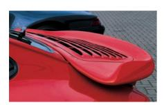
The 993 Turbo featured the traditional tea-tray rear wing—necessary to accommodate the twin intercoolers in the engine compartment—but with downturned side fences.
