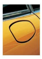
A 1972 model 2.4 can be identified by the oil filler flap on the right-hand rear wing—where it remained for only one year. Placing the oil tank within the wheelbase helped the handling, but this arrangement proved to be impractical because filling station attendants sometimes put petrol in the oil tank.
