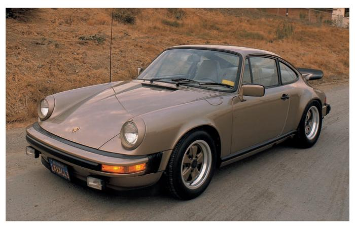
Weissach models were available in Black Metallic or, as here, Platinum Metallic. The centers of the Fuchs alloy wheels were colorcoded to the body. 16-inch diameter forged-alloy Fuchs wheels with Pirelli P7 tires, sizes being 6J wheels with 205/55VR tires at the front and 7J wheels with 225/50VR tires at the rear. These sizes were an option in other markets. The Fuchs wheels of the 1982 models had highly polished rims with black gloss centers.
