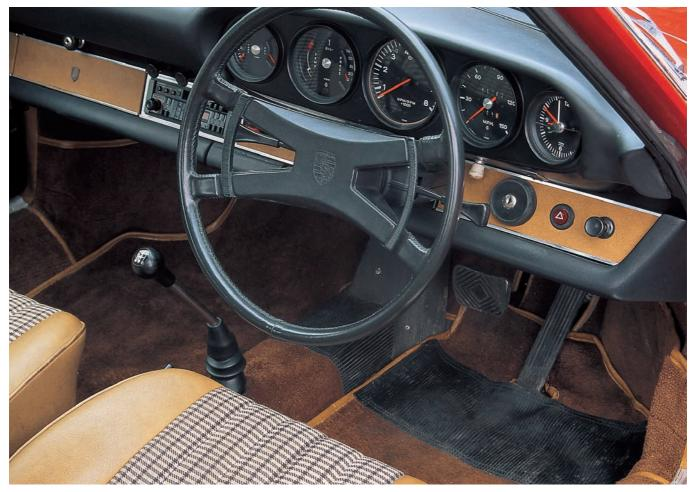
Nancy MacLean's smart 1973 Sportomatic (above) has a two-pedal arrangement and a conventional-looking gear lever (top right). Porsche's automatic was quite different from any other manufacturer's. There was no clutch, but the driver still changed gears by moving the lever through a conventional gate. The Sportomatic's popularity waned through the 1970s.
