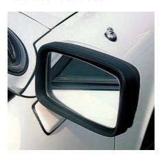
Large exterior mirrors were introduced in 1976. The body of the mirror was color-coded, while the mirror itself was electrically adjustable and heated.
