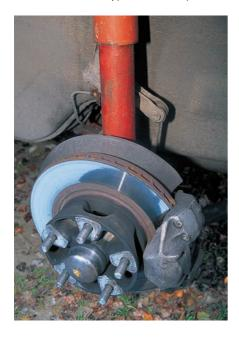
The front suspension of an early 911S shows off a red Koni strut and ventilated disc with the M-type cast-iron caliper. The A-program S model received a dual-circuit braking system, a safety factor that helped to cure the earlier tendency for the car to pull to one side under braking, and the B-program S was given light alloy S-type front calipers.
