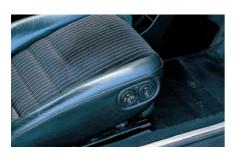
The seats on the Carrera 3.2 have electric adjustment for height, cushion angle, and recline, with this control panel set on the side of the cushion.
