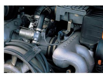
Digital Motor Electronics came to the 911 for the 1984 model year, improving performance and reducing fuel consumption by 10 percent.
