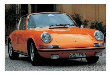
A very clean 1971 2.2 Targa. Ventilation on the Targa had been improved for the 1969 model year by the addition of vertical cabin air outlets at the sides of the roll-over hoop. Although deleted from the coupe, the opening front quarter lights were retained on the Targa until 1977. Not often seen today is the "Weltmeister 1969/70" decal in the left lower area of the windshield, celebrating the factory's consecutive World Championship of Makes racing titles.
