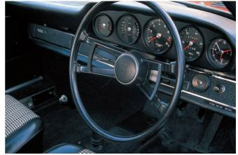
The markings of the dials changed from green to white for the 1968 model year, and chrome trim virtually disappeared from the dashboard. Interesting details include the large switch under the clock for the optional sunroof and the heavy grain lower dash that was also new for the 1968 model year.
