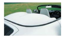
The Speedster's large fiberglass hood cover molding hinges backward and remains in place all the time, precluding the fitting of rear seats.
