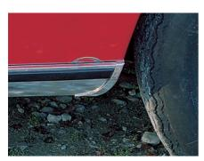
The sills of the 911S featured deeper aluminum trim extrusions and "wide" rubber trim. Peeping out from behind the trim is the circular torsion bar cover. The short-wheelbase 911s, built to the end of the 1968 model year, are visually identified by the closeness of the cover to the wheel arch
